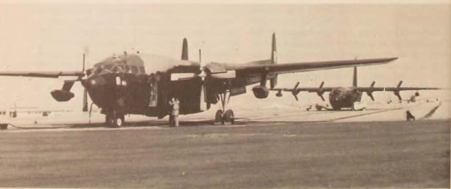
The AC-119K gunship's two added J-85 jet pods increase its load capacity and single-engine performance.
